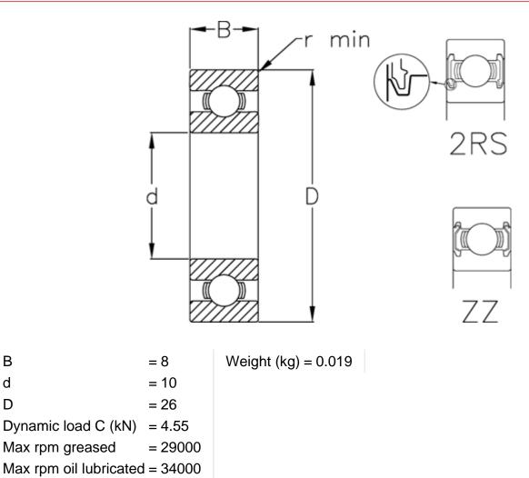
r min = 0.3 Static load C0 (kN) = 1.96
